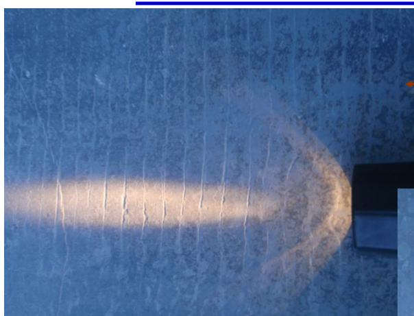
Casting at a lower frequency of oscillation for the mold enforced by simple proportional controllers
